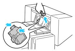
4. Hold the tabs on both sides of the new staple cartridge and insert it into the original position in the finisher.
