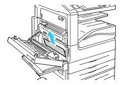
3. Open the fuser by pulling out the handle labeled A1.
