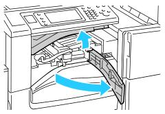
2. Pull out the hole punch waste container.
