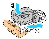
7. Grip the staple cartridge by the orange handle and insert it into the stapler assembly. Push it in until it clicks
