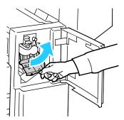
4. Grip the staple cartridge by the orange handle and pull it firmly toward you to remove it. Check inside the finisher for any loose staples and remove them.
