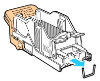
8. Push the clamp in the direction shown until it snaps into the locked position.
