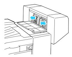
3. Hold the tabs on both sides of the staple cartridge and pull the cartridge out of the finisher.
