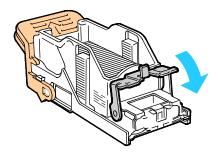
9. Grip the staple cartridge by the orange handle and insert it into the stapler assembly. Push it in until
