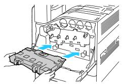
9. Rotate the waste container up, toward the printer until it clicks into place.
