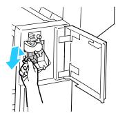
5. Pinch both sides of the staple pack (1) and remove the staple pack from the cartridge (2).
