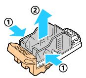
6. Insert the front side of the new staple pack into the staple cartridge (1), then push the rear side into the cartridge (2).
