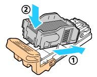
6. Grip the staple cartridge by the orange handle and insert the cartridge into the stapler until it clicks.
