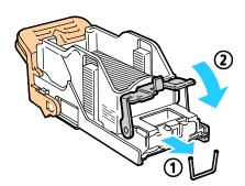
5. Grip the staple cartridge by the orange handle and insert the cartridge into the stapler until it clicks.
